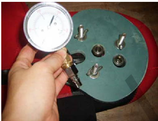
7. Check the operational condition of pressure gauge (Dial surface & Pointer).
