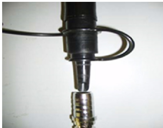
10. Adjust the multi-valve adaptor on the connector of face fixture.
