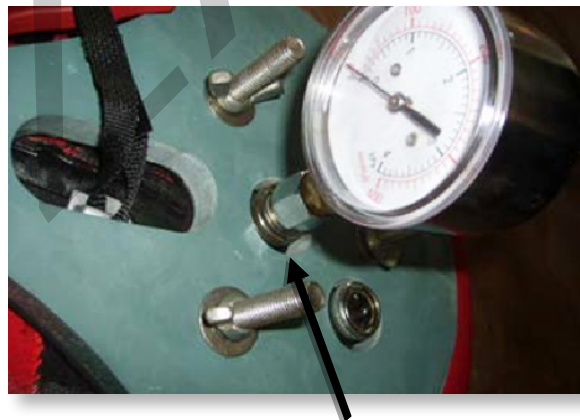
8. Insert the Pressure Gauge at face fixture socket, at the same time press down the joint and secure the connection between them.
